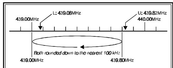
*For the purposes of PMS scanning, the operating mode and synthesizer steps programmed into the frequency associated with the “L” memory slot will be utilized.*
