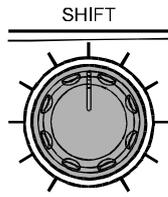
The **SHIFT** control's 12 o'clock (center) position represents the "normal" passband center frequency. Rotate the **SHIFT** control to the left or right to eliminate interference. Careful adjustment of the **SHIFT** control may also be useful in improving the recovered audio on excessively bassy SSB signals. Return the **SHIFT** control to the center position to return to the normal default passband setting.
