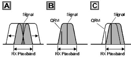
This feature is operational in all modes except FM, although the effect in the AM mode may not be dramatic due to the wider bandwidth used during AM operation. The **SHIFT** control's function is dedicated to the receive mode, and does not affect your transmitted signal characteristics; such adjustment of the transmitted signal is, however, provided via Menu items #92 and 93, as described on page 90.
